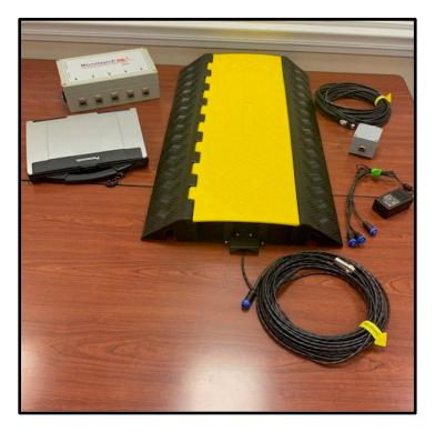
Standoff Vehicle Sensor is imbedded in speedbump
