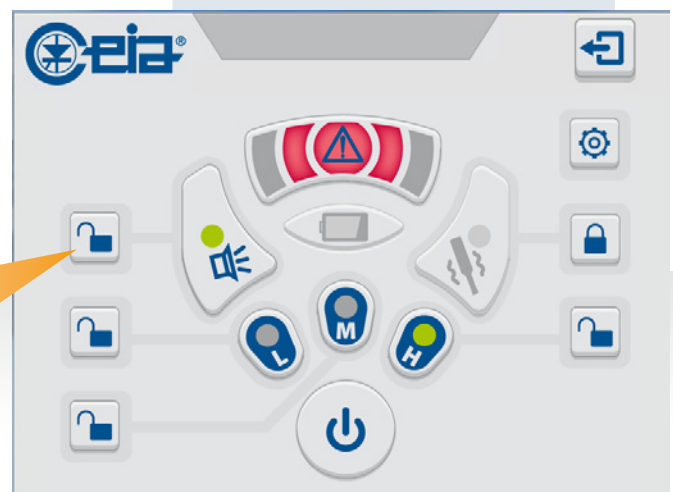
Optical indication proportional to the metal signal strength [Low, Medium, High]
